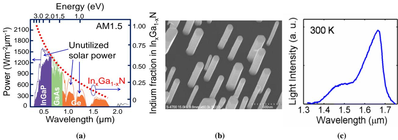
**Fig. 20.** (a) The utilized solar power spectrum of a triple junction Ge/GaAs/InGaP solar cell and bandgap energies of the InGaN alloy system that cover the entire AM1.5 solar spectrum; (b) SEM image of non-tapered InN nanowires grown directly on Si substrates; (c) photoluminescence emission spectrum measured at room-temperature.
