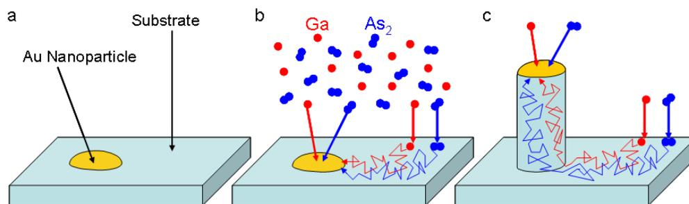
**Fig. 19.** Illustration of typical nanowire growth process. (a) Metal nanoparticles (typically Au) on a substrate surface. (b) Precursor gas atoms and/or molecules (e.g., Ga, As<sub>2</sub>) are incident on the substrate surface, diffuse and become trapped by the metal particle. (c) Supersaturation of the metal particle results in the formation of a nanowire (GaAs in this case).
