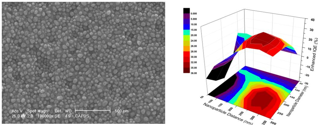
Figure 4. Silver nano-island fabrication after thin film deposition and nanofabrication on glass coated with sputtered AZO (left) and Internal Quantum Efficiency (IQE) silver nano-island on top of proposed nc-Si:H solar cell as a function of different parameters, through FDTD simulation (right).
