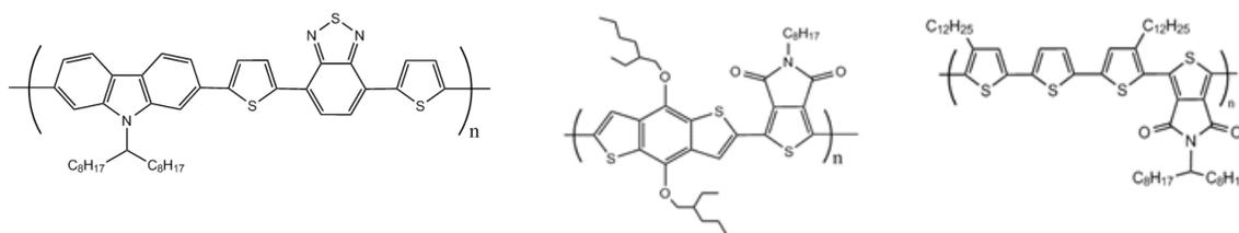
Figure 6. Chemical structure of PCDTBT (left), PBDTTPD (middle) and AP079 (right).
