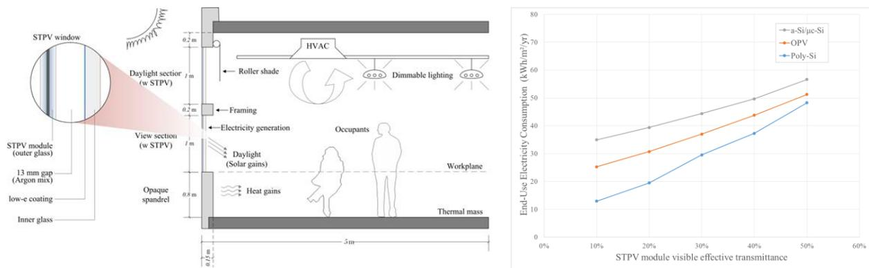
Figure 1. A schematic of major interactions between the STPV windows, the office space and the occupants (left) and the annual end-use electricity consumption of three STPV cell technologies (right),
