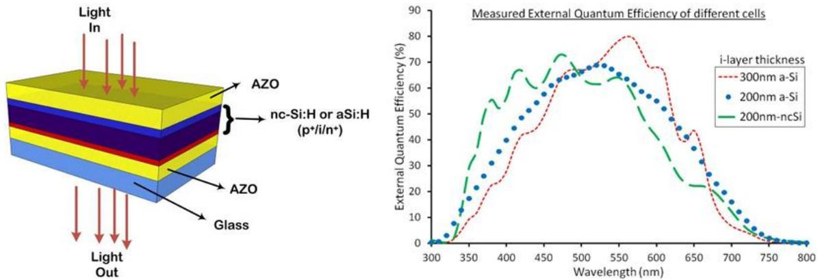
Figure 3. Schematic of the Glass/AZO/a-Si ( $n^+/i/p^+$ )/AZO solar cell structure on glass (left) and EQE of developed cell with 200nm nc-Si in compare to previously developed 300nm and 200nm a-Si absorber layer (right).
