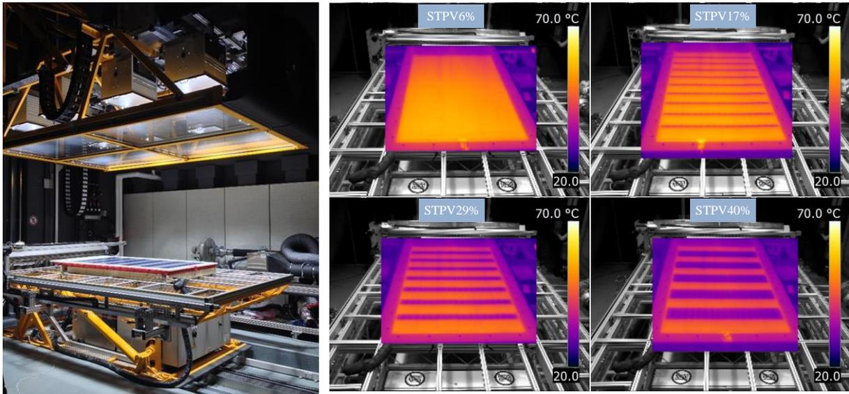
Figure 2. STPV window tested under the Concordia University solar simulator laboratory (left) and temperature profile for four STPV prototype windows, under 1000W·m<sup>-2</sup> and ambient air temperatures of 21°C (right).
