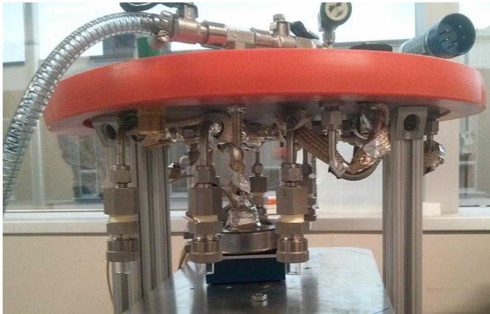
Fig. 5 System for vapour-phase deposition of conductive polymers
