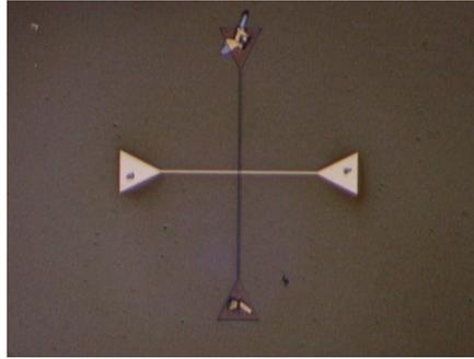
Fig. 4 SEM of Cross-Bridge Kelvin Resistor geometry used to measure through-post conductivity.
