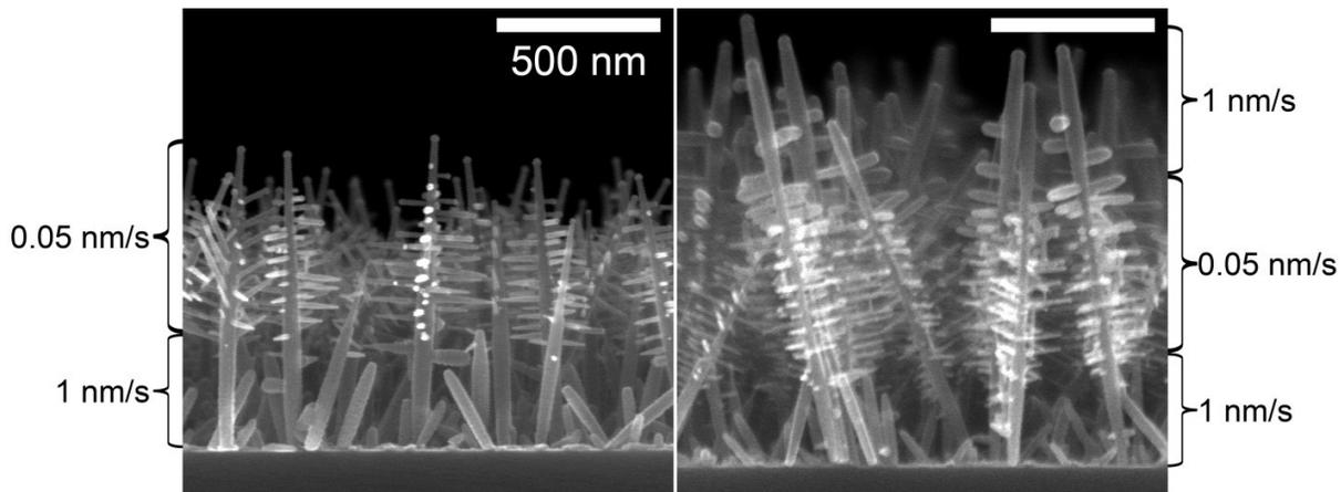
Fig. 2 Indium tin oxide trunks and branches grown by GLAD-moderated VLS. Branching is controlled by the deposition rate (relative to spin speed) indicated on the figure.
