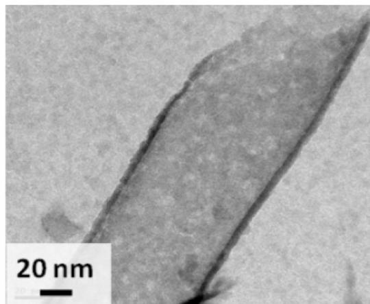
Fig. 1 TEM image of silicon nanotube with  $\approx 6$  nm wall thickness.
